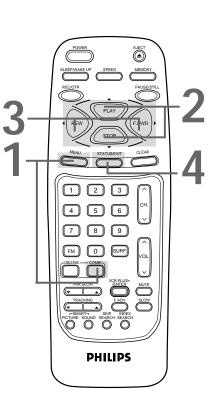
Press the REW(ind)/◀ button or the F.FWD/► button to select ON or OFF. Each press of the REW(ind)/◀ button or the F.FWD/▶ button turns REMINDER ON or OFF.
